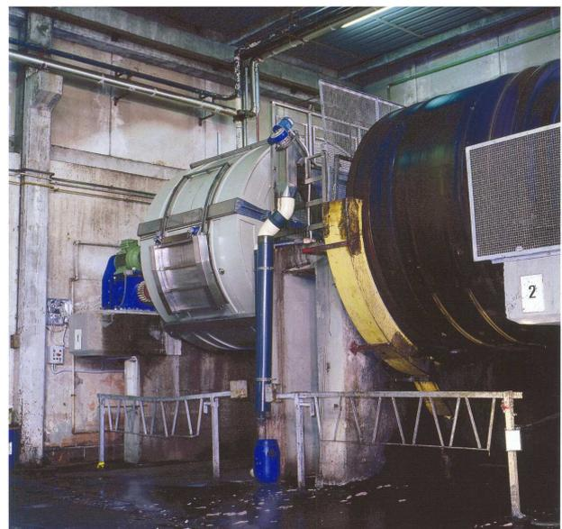
Picture. 1 - Polypropylene and Wooden drum running side by side
