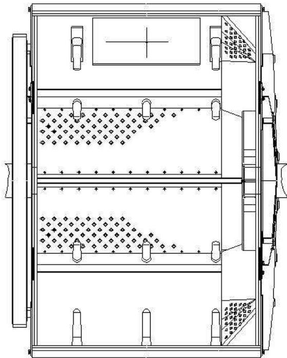
Picture 2: Polypropylene drum section
