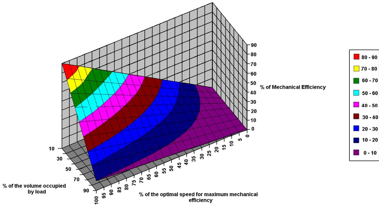
Picture 10 : Efficiency of an ideal drum.
