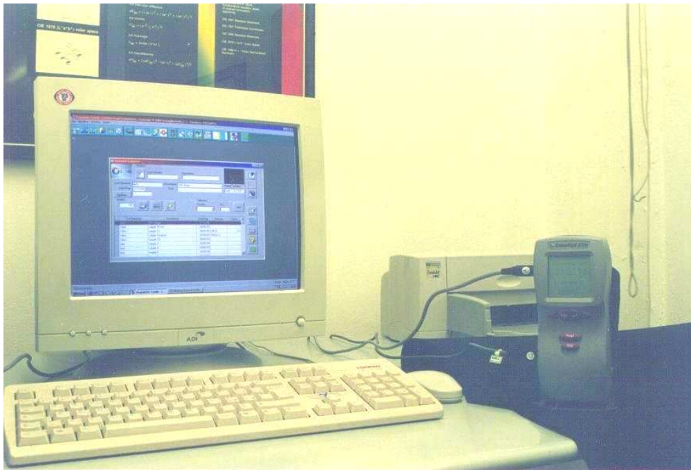
Picture 5: Samples measurement with Colour Eye ETH Spectrophotometer.
